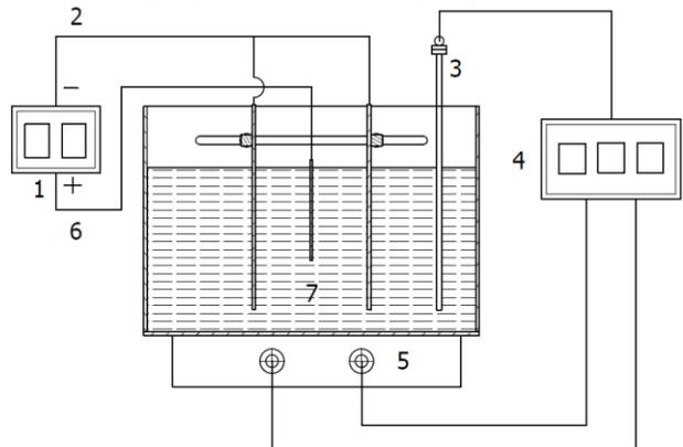
Figure 4: The schematic diagram of the improved electropolishing device's working principle.
