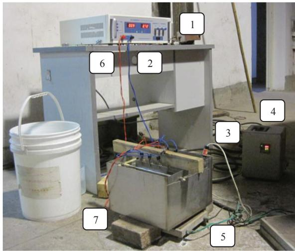
Figure 5: Photo of the improved electropolishing device
