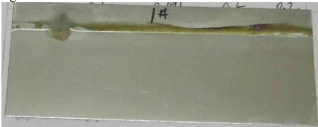
Figure 3: The photo of the tungsten sheet after electropolishing
