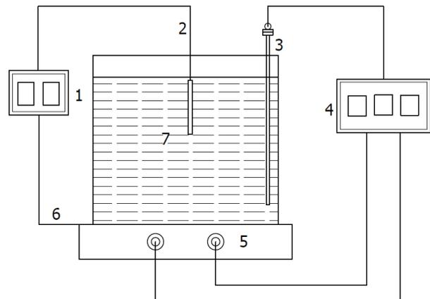
Figure 1: the schematic diagram of the electropolishing device's working principle.
