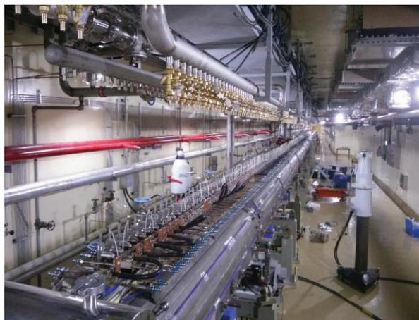
Figure 5: DTL tanks were aligned in the tunnel by using two laser tracker systems. The position was monitored in real time.
