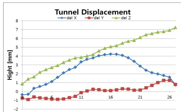
Figure 3: Tunnel displacement according to the increasing of the temperature as 20 °C.
