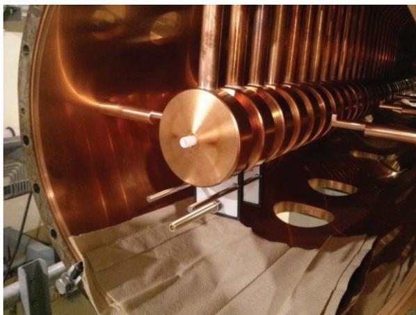
Figure 4: The position of drift tubes were checked and realigned.
