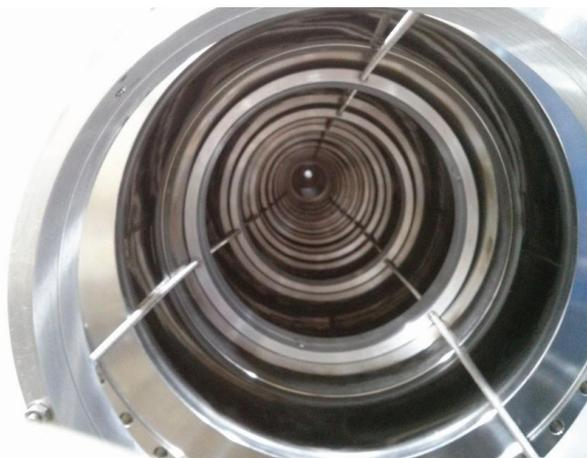
Figure 6: Collimators inserted in the beam pipe.
