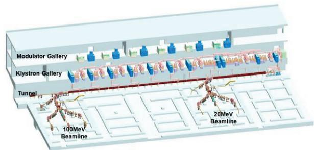
Figure 1: The layout of the linac, beam lines and the accelerator building.
