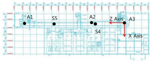
Figure 2: Coordinate system for the accelerator. The coordinates of A1 and A3 are linked with the coordinate system used for the construction.
