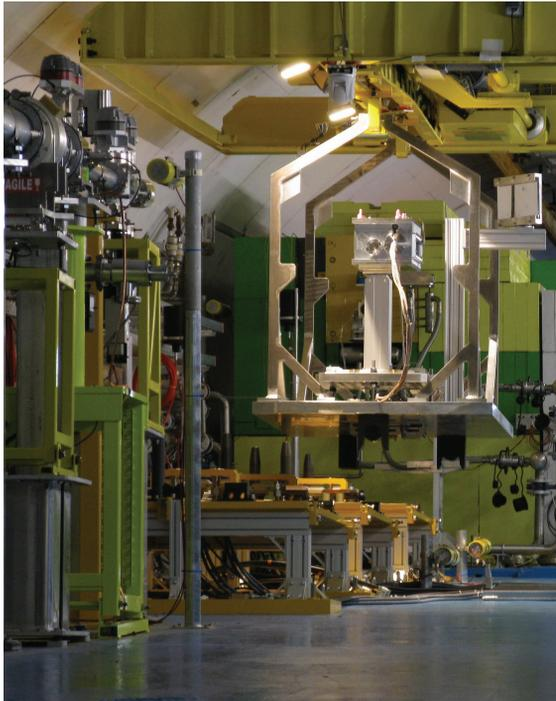
Figure 3: The remote installation of the HRMT10 experiment on the target position. In the left foreground the primary beam vacuum pipe is visible. The picture background shows the beam dump. On the right side of the trough setup one can see mirrors, which guided the light of the high-speed camera and the laser-Doppler vibrometer.
