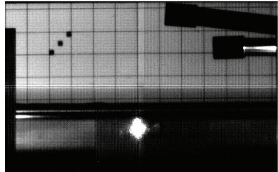
Figure 4: One frame as recorded by the optical observation system (before beam impact): The upper surface of the powder is located at the lower edge of the 1-cm grid. The beam direction is from the left. The bright spot in the lower part of the image is caused by the LDV laser beam, pointed at the trough.
