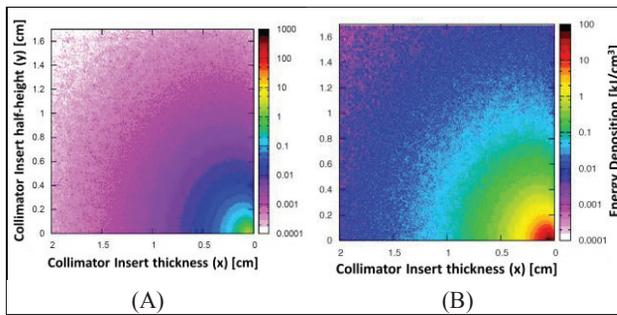
Figure 2: Energy deposition cuts in the x-y plane at the location of  $T_{\max}$  in z. (A) 1 nominal bunch of lead ions ( $7 \times 10^7$  ions, 2759 GeV/n) with  $T_{\max}$  occurring at  $z = 6.5$  cm. (B) 1 nominal bunch of protons ( $1.15 \times 10^{11}$  p) at 7TeV with  $T_{\max}$  occurring at  $z = 7$  cm.
