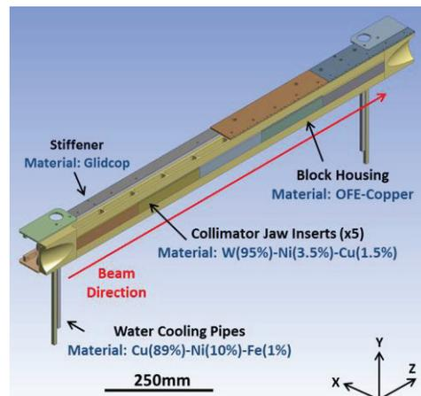
Figure 1: Left jaw assembly of a TCH.
