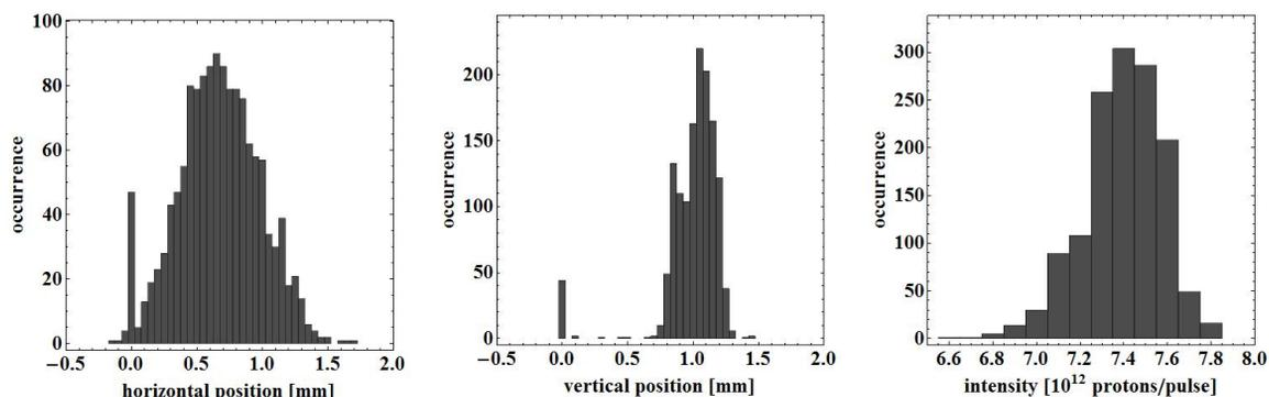
Figure 4: Beam position and pulse intensity stability during a 48 hour run (1500 extractions) for the HRMT01 experiment. The beam position has a  $\sigma$  of 0.3(0.1) mm in the horizontal(vertical) plane, and the beam intensity is stable to 1% level.
