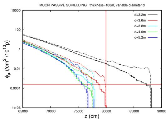
Figure 5: Muon fluxes downstream the hadron stop for various diameters of a 100 m long iron shielding. The full lines correspond to the total flux over a  $5 \times 5 \text{ m}^2$  area, whereas the dashed lines to the maximum value in the same area. The horizontal line is the acceptable muon rate limit, and the vertical line the foreseen location for the near detector.
