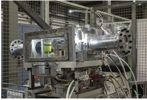
Figure 1: Photo showing the aluminium box containing the crystal. Photo by courtesy of Maximilien Brice.
