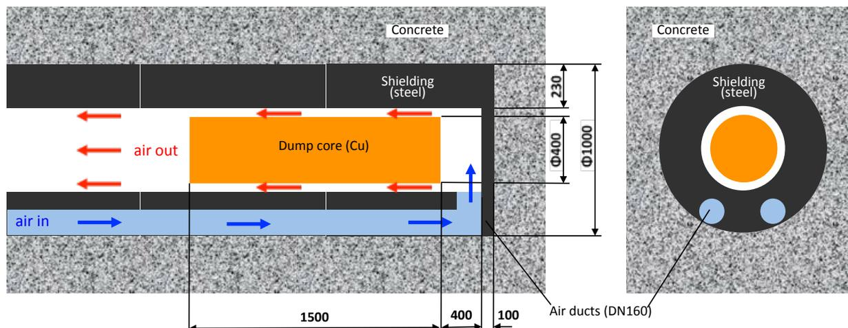
Figure 3: Proposed design for new dump-shielding assembly
