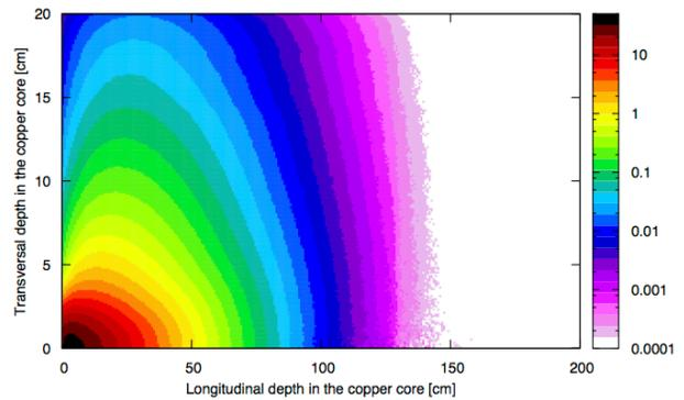
Figure 2: Energy deposition inside dump (GeV/cm<sup>3</sup>)
