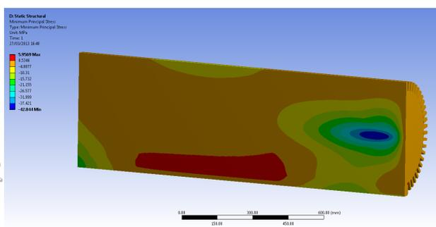
Figure 5: Compressive stress distribution at steady state.
