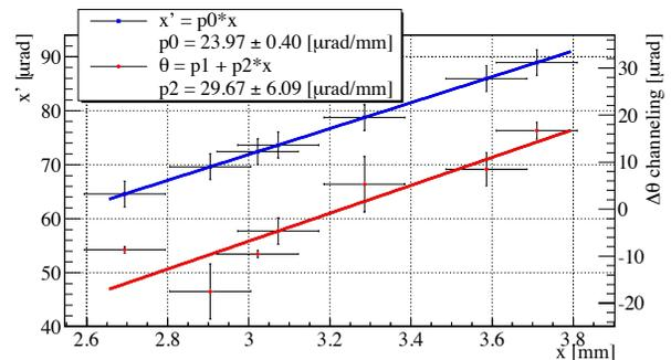
Figure 1: Theoretical beam divergence (left scale, blue line) as a function of the crystal distance from the closed orbit ( $x$ ), and measured channeling orientation from a reference angle (right scale, red line).
