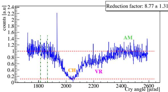
Figure 5: Example of the losses seen by the BLM in the high dispersive area during an angular scan.
