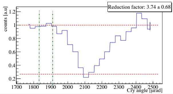
Figure 6: Example of the losses seen by an SPS-BLM in the sextant 4 (BLM 420), during an angular scan with a crystal placed in the sextant 5.
