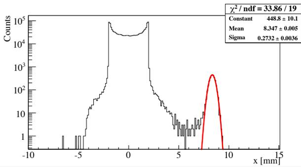
Figure 2: Simulated particles distribution at the Medipix location: beam core around 0, channeled and extracted beam around 8.4mm.
