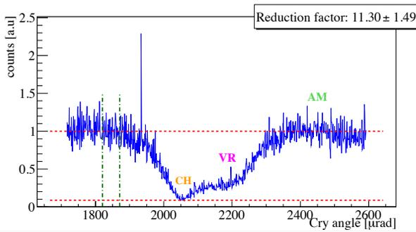
Figure 4: Example of the losses seen by the BLM close to the crystal during an angular scan.
