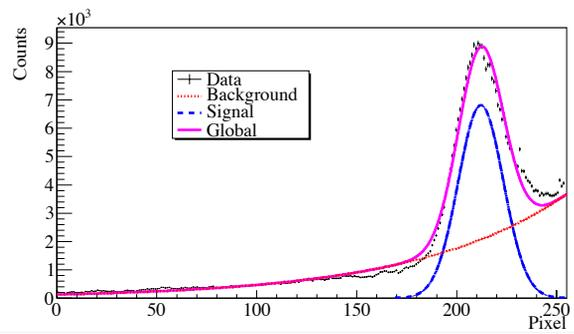
Figure 3: Horizontal projection of the experimental spot of the channeled and extracted beam, seen by the Medipix.
