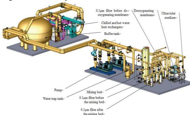
Figure 5: Process of DIW treatment.
