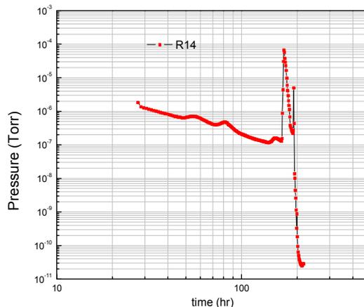
Figure 6: TPS, one cell pumping curve
