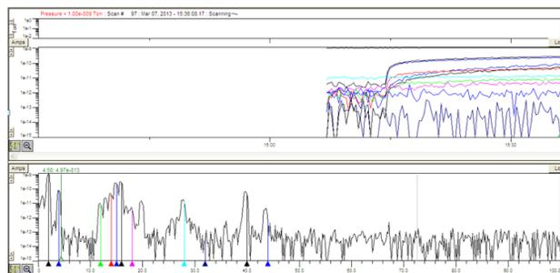
Figure 7: Spectrum of residual gases
