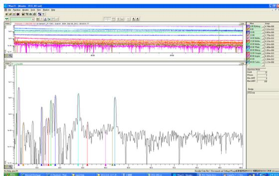
Figure 4: RGA spectrum in IU after decreasing the temperature for 24 hours.
