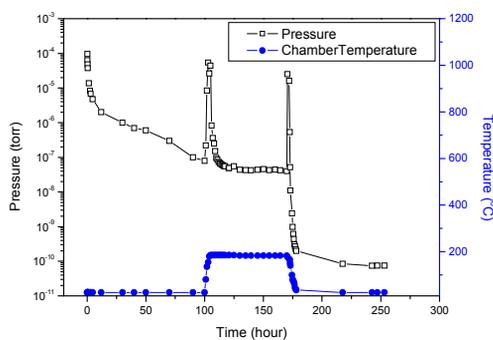
Figure 1: Pumping curves for IU vs time during a baking test.
