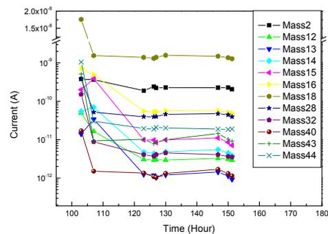
Figure 3: Residual gas during baking test at 180 °C (the chamber temperature).
