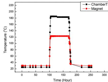
Figure 2: Baking temperature of the main chamber and magnet arrays in IU vs time.
