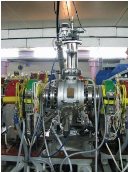
Figure 4: NESTOR RF cavity installed in the ring.
