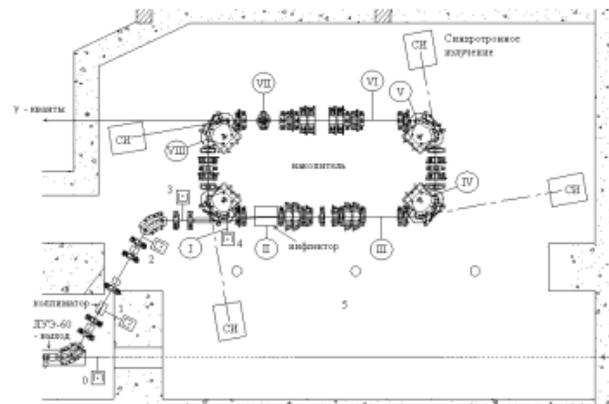
Figure 1: The lattice of X-ray generator NESTOR injection channel and storage ring with layout of vacuum system.
