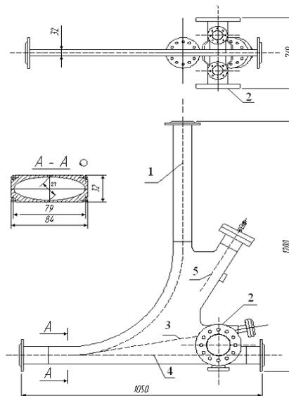
Figure 2: Dipole magnet vacuum chamber drawing.
