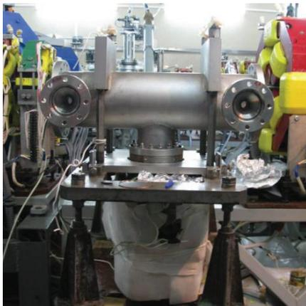
Figure 5: NESTOR inflector vacuum chamber before installation.
