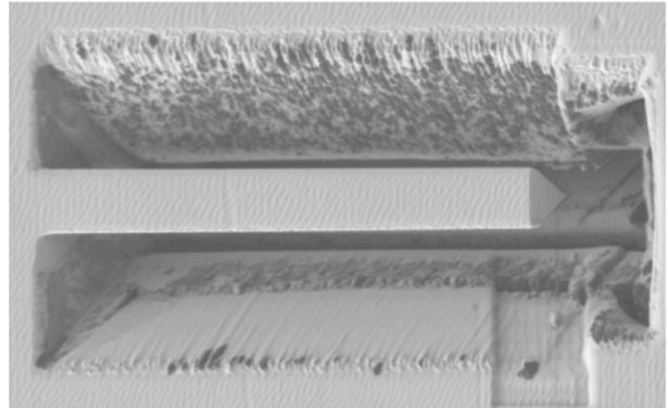
Figure 3: Micro-cantilever ( $17\mu\text{m} \times 3\mu\text{m}$ ) machined in tungsten (image courtesy of D. Armstrong, Oxford).
