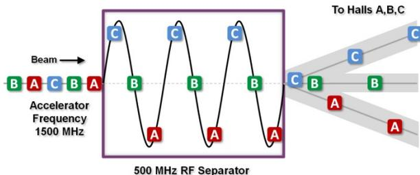
Figure 4: 500 MHz separation triple split for fifth pass (not to scale).
