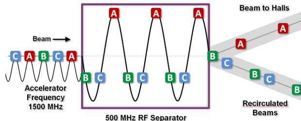
Figure 3: 500 MHz separation to kick one out and recirculate two (not to scale). This is the configuration for the first four passes.
