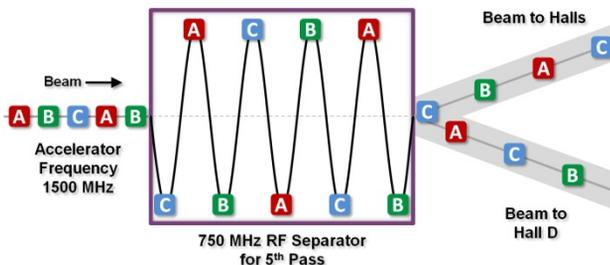
Figure 6: 750 MHz separation with all buckets filled (not to scale).
