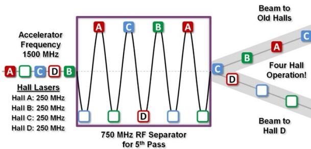
Figure 7: Proposed 750 MHz separation for four hall operation (not to scale).
