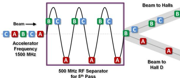
Figure 5: 500 MHz 5<sup>th</sup> pass separation for three-hall operation (not to scale).
