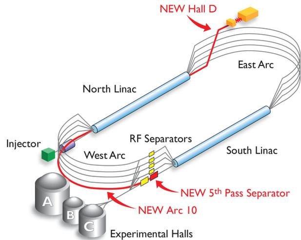
Figure 1: Layouts of 6 and 12 GeV CEBAF. The 12 GeV transport lines added to support the new experimental hall, Hall D, are shown in red.
