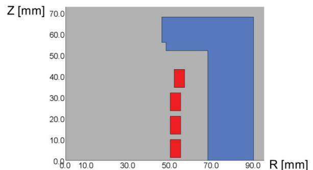
Figure 2: Opera 2D cross sectional view of the axisymmetric solenoid model. The HTS coils are shown in red, and the iron yoke is shown in blue.
