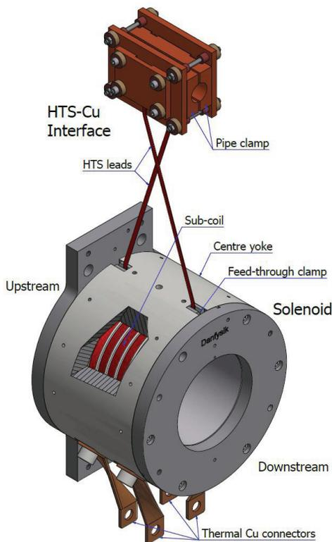
Figure 3: Schematic view of the solenoid.
