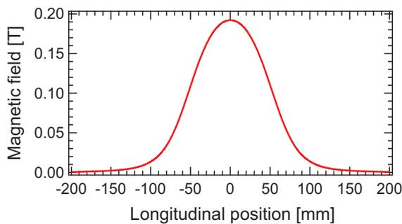
Figure 4: Plot of the axial magnetic field measured along the solenoid axis.
