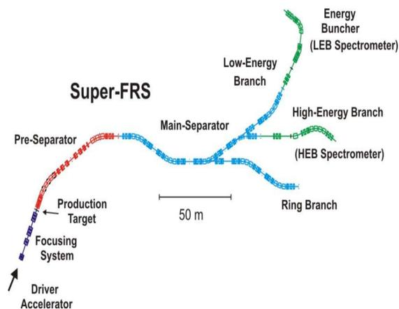
Figure 1: Layout of Super-FRS.
