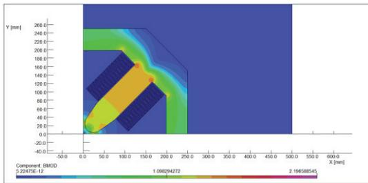
Figure 2: Magnetic flux density distribution.
