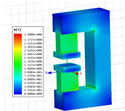
Figure 3: The magnetic flux distribution on the surface of yoke and pole head.
