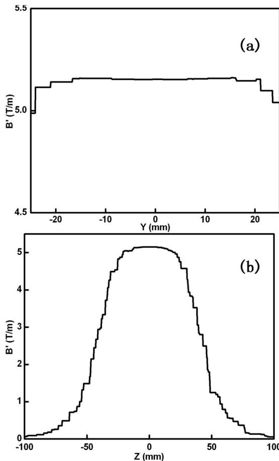
Figure 8: The distribution of magnetic field gradient  $B'$  along Y axis (a) and Z axis (b).
