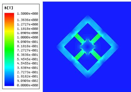
Figure 7: The distribution of magnetic flux on XY cross section of quadrupole.
