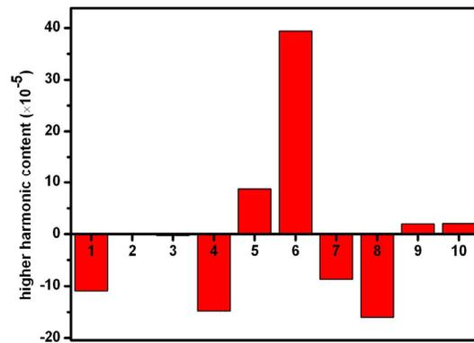
Figure 9: Higher harmonic content of magnetic field of quadrupole.
