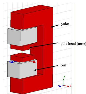
Figure 2: The magnetic model of dipole.
