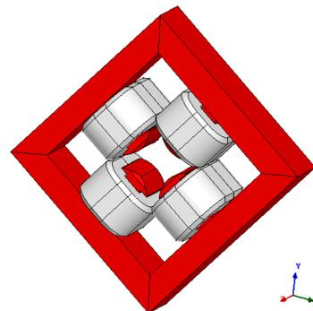
Figure 6: The magnetic model of quadrupole.
