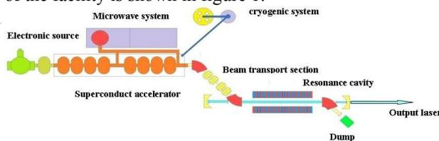
Figure 1: The layout of THz FEL at CAEP.
