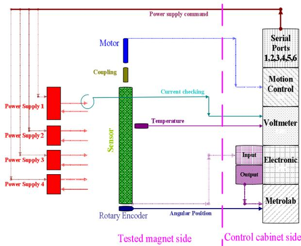
Figure 2: Measurement coil schematic diagram.
