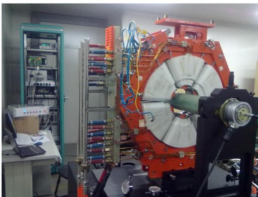
Figure 3: The photo of new harmonic coil bench.
