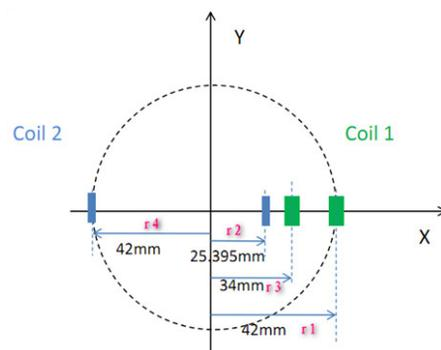
Figure 1: Measurement coil schematic diagram.
