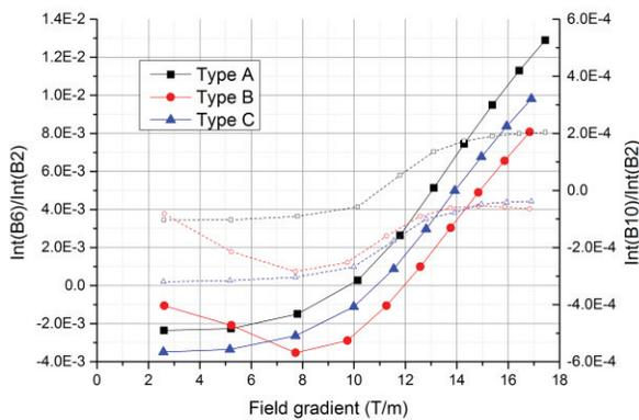
Figure 6: The ratios of integrated dodecapole field (solid line) and 20-pole field (dashed line) to integrated quadrupole field.
