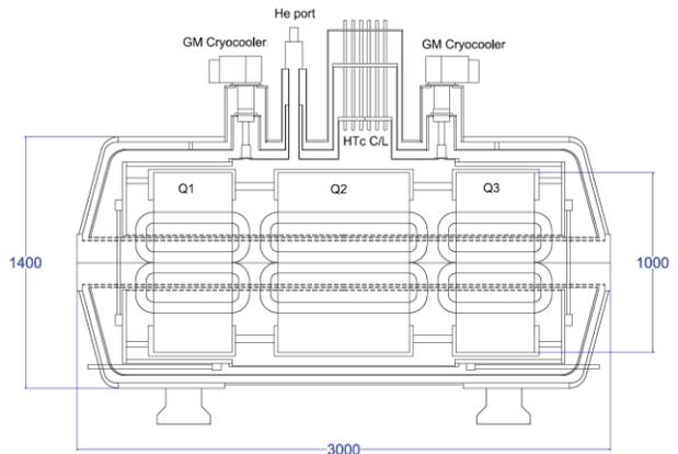
Figure 4: Schematic sectional view of the cryostat with a prototype of superferric quadrupole magnet triplet inside.
