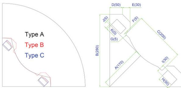
Figure 5: Quadrant cross section of three types of quadrupole magnet (left) and the pole geometry of type B (right).
