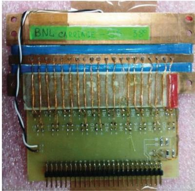
Figure 2: Hall probe array.
