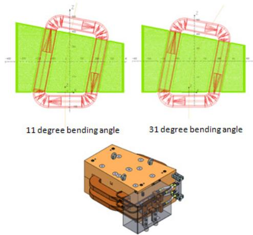
Figure 1: The yellow line shows the electron beam trajectories for 11° and 31° operation of the LTB dipole magnet. An engineering drawing is below.
