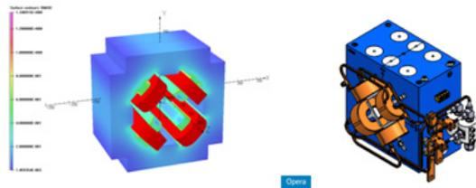
Figure 2: The model (Opera 3D) is shown at the left; an engineering drawing of the LTB quadrupole magnet is shown at the right.
