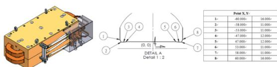
Figure 4: Pole profile points of the BTS dipole magnet
