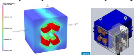
Figure 5: Model (Opera 3D) is shown at the left, and an engineering drawing of the BTS quadrupole magnet at the right.
