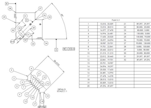
Figure 3: Pole profile points of the LTB quadrupole magnet.
