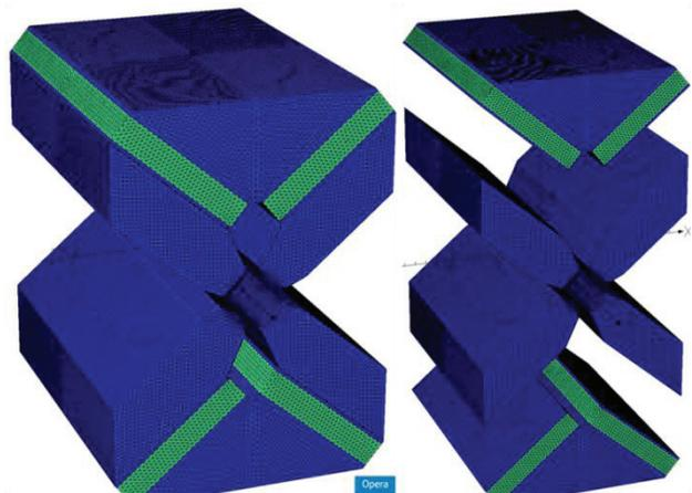
Figure 2: A 3D representation (using Opera) of the design of the high-strength quadrupole.
