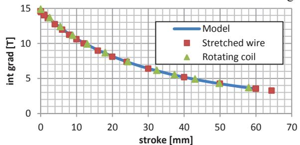
Figure 5: Integrated gradients measured at CERN, compared with the 3D model.
