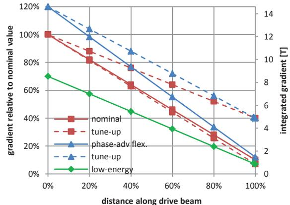
Figure 1: Tuning range required for DBD quadrupoles.
