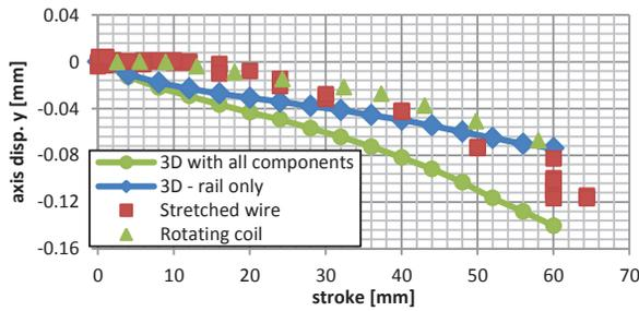
Figure 6: Measured axis displacements, showing comparisons with modelled values.
