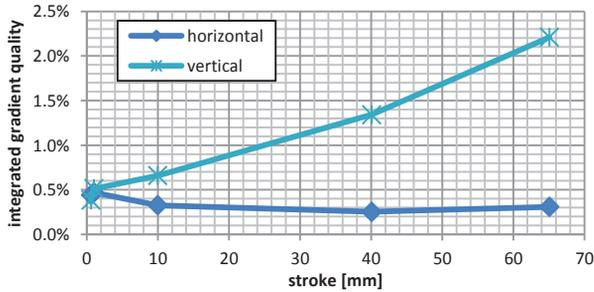
Figure 7: Measured values of integrated gradient quality over the 23mm aperture.
