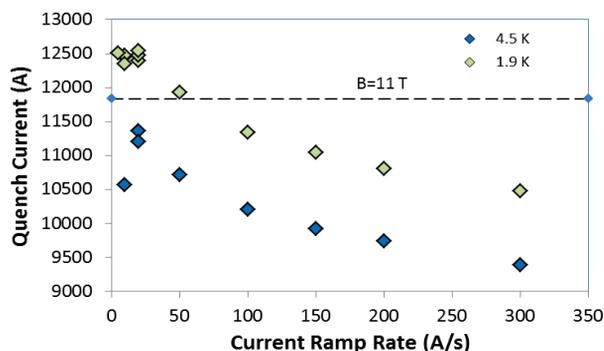
Figure 6: Ramp rate sensitivity of magnet quench current.
