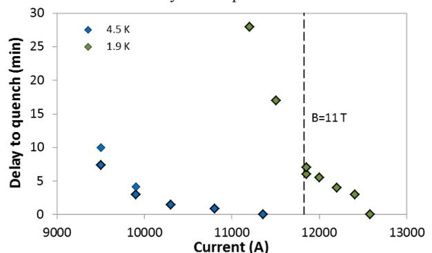
Figure 5: Holding time to quench vs. plateau current.
