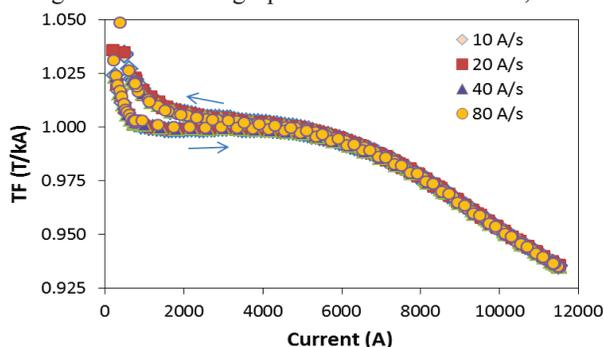
Figure 8: Transfer function  $TF$  vs. magnet current.
