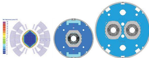
Figure 1: The 2-layer coil (left), single-aperture (middle) and twin-aperture (right) dipole cold masses. The dark area in the coil bore corresponds to relative field errors below 10<sup>-4</sup>.
