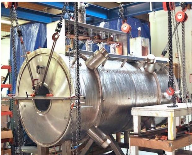
Figure 6: Second spectrometer solenoid nearly completed.
