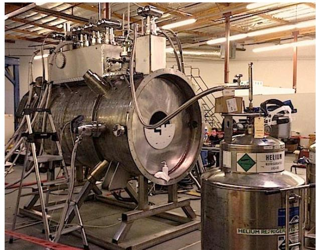
Figure 2: First spectrometer solenoid during training.
