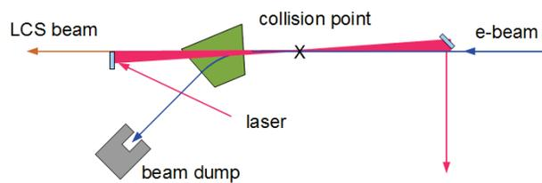
Figure 3: Layout of laser Compton scattering.
