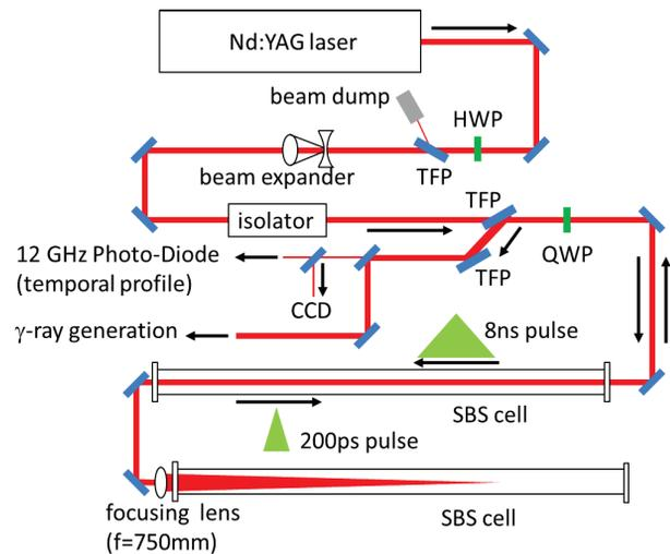
Figure 4: The laser system for  $\gamma$ -ray generation.
