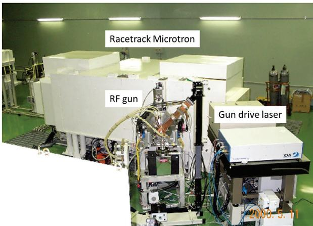
Figure 2: The 150-MeV racetrack microtron.
