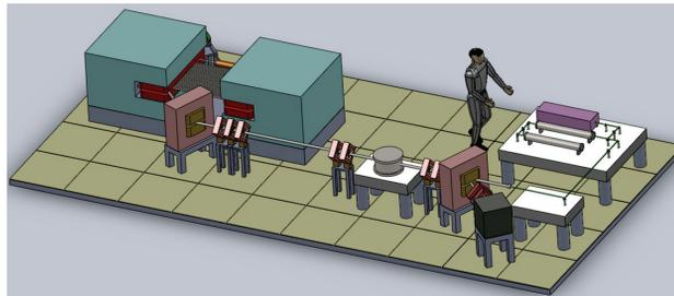
Figure 6: Conceptual design of a 1.7-MeV  $\gamma$ -ray source based on a 220-MeV racetrack microtron and a frequency-doubled Nd:YAG laser.
