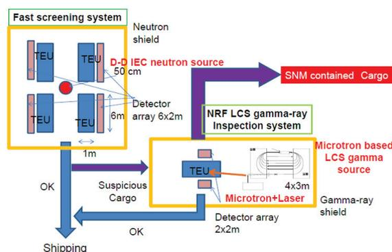
Figure 1: Conceptual design of the inspection system for nuclear material.
