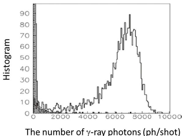
Figure 5: Histogram of  $\gamma$ -ray photon statistics obtained from the direct method. The number of photons per shot is  $(6.3 \pm 1.5) \times 10^3$  ph/shot. The hatching area is a histogram without the laser pulse injection as a background signal.
