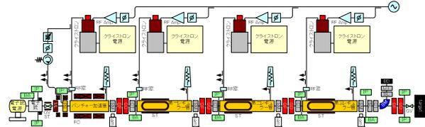
Figure 8: Layout of 60 kW 30 MeV S-band Linac for On-site Neutron Active Method Analysis in Fukushima.
