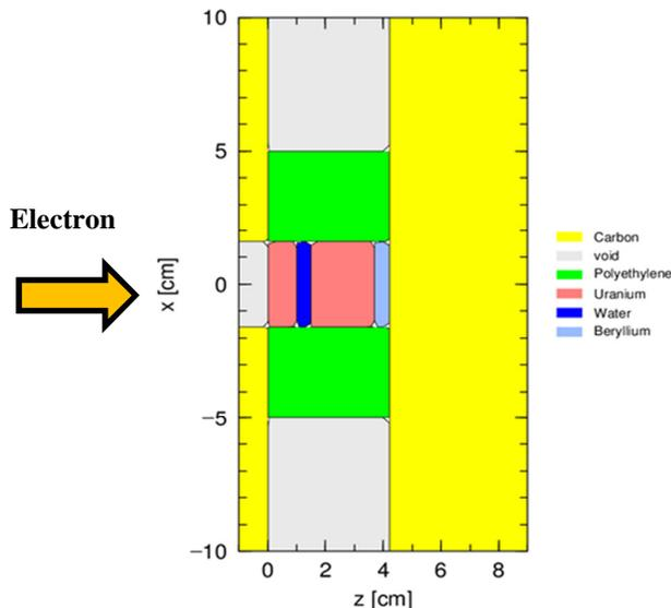
(a) Cross Section of the NeutronTarget
