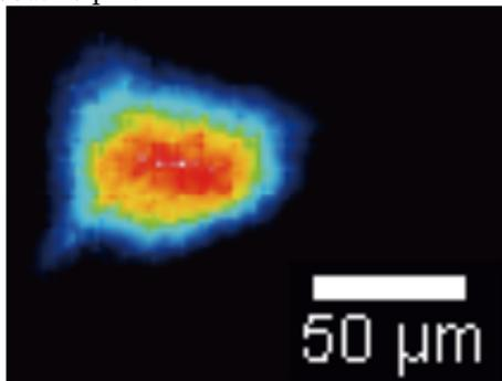
Figure 7: The focused beam profile measured by GAFCHROMIC FILM.
