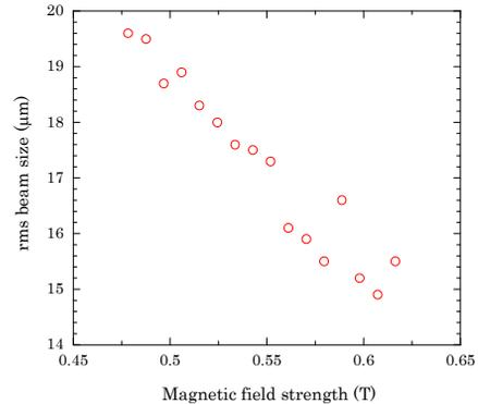
Figure 4: Simulated dependence of rms beam size on magnetic field strength of solenoid lens 2.
