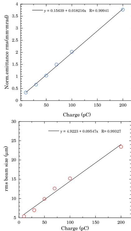
Figure 5: Simulated the dependence of normalized emittance (upper plot) and rms beam size on charge of electron beam (bottom plot).
