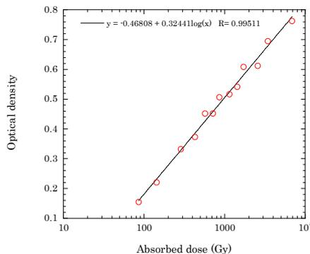
Figure 6: The calibration curve of HD-810 film.
