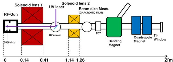
Figure 2: Schematic design of beamline.
