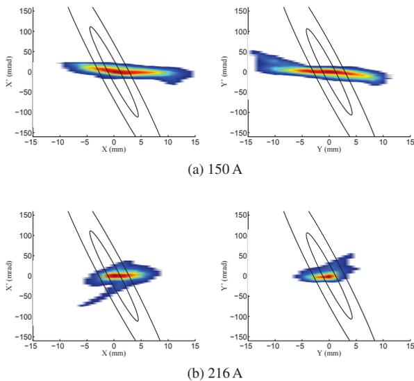
Figure 6: Horizontal and vertical emittance measurements at the LEBT exit for different currents in the final LEBT solenoid. Also shown are 100% emittance ellipses for  $0.25\pi$  and  $1.5\pi$  for the matched Twiss parameters.
