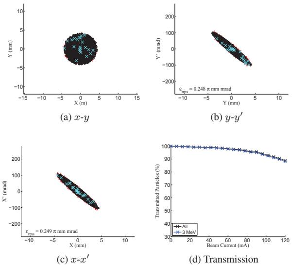
Figure 1: RFQ transmission and input beam distributions for design input parameters and emittances (see main text). Input distributions are coloured according to particle survival: black are transmitted to 3 MeV, red are lost and blue transmitted but not correctly accelerated.
