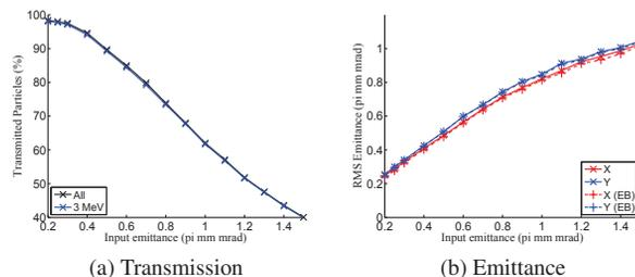
Figure 3: Transmitted current and emittance as a function of input emittance for the matched Twiss parameters. Exit emittance measured at a fixed point in time is marked “EB”.
