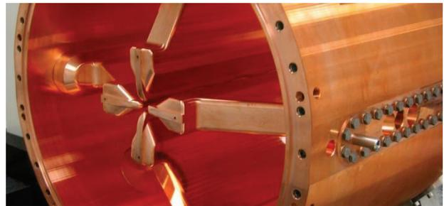
Figure 4 : RFQ end-vane details.
