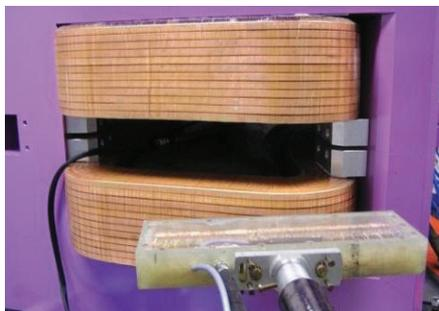
Figure 5 : Field measurements of HEBT dipole magnets.
