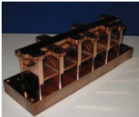
Figure 2: The four-rod model of the FAIR proton linac RFQ.
