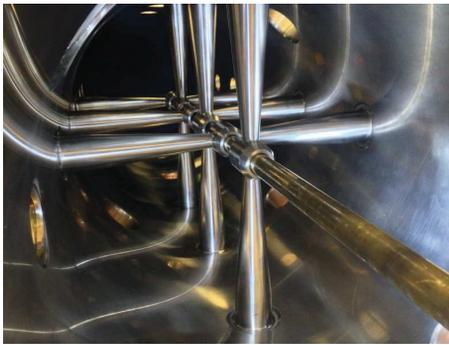
Figure 6: The stainless stems welded into the outer cylinder.
