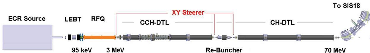
Figure 2: The schematic layout of the FAIR proton linac including the position of the XY steering magnets.
