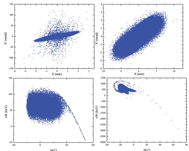
Figure 1: On the left side the horizontal and vertical RFQ output distribution, on the right the corresponding distribution at the DTL exit. Non accelerated particles are shown only in the transversal plane.
