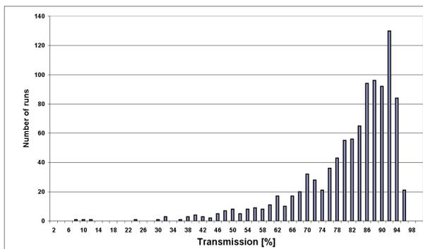
Figure 5: Statistical analysis of the transmission over 1000 runs.
