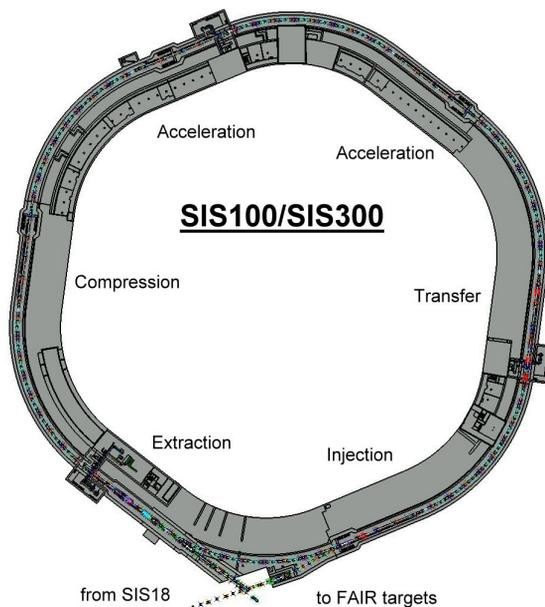
Figure 1: SIS100/300 accelerator tunnel with its parallel supply tunnel. Indicated are the main functional sections of the six SIS100 straights. The three niches (down left and right and up) comprise the local cryogenics system of SIS100. One further niche in the north is foreseen for a later set-up of a laser cooling system.
