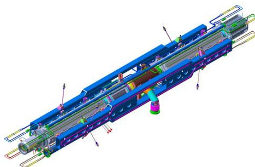
Figure 4: Design of the cold mass of the SIS100 quadrupole module. Two quadrupole magnets and corrector magnets (steerer and sextupole) are installed on a common girder. In between the quadrupole magnets, a cryogenic ion catcher is mounted. The catcher chamber will also be used for roughing the UHV system. A BPM is attached to the yoke of the first (left) quadrupole magnet. The module accommodates the s.c. bus bar system of the dipole and of three quadrupole circuits.
