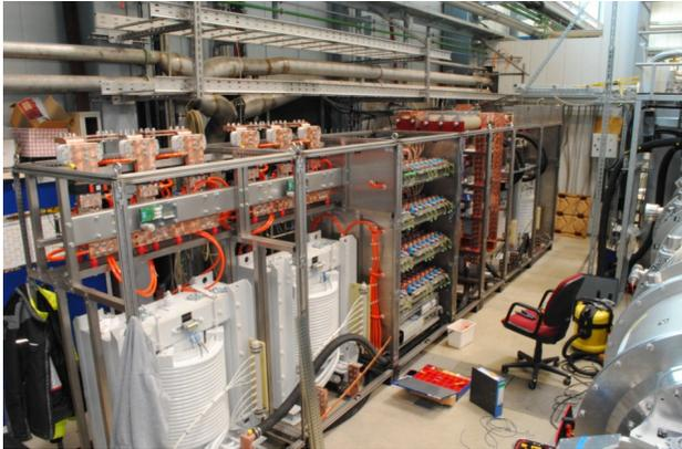
Figure 5: 20 kA power converter upgrade for the existing superconducting magnet test stand at GSI.
