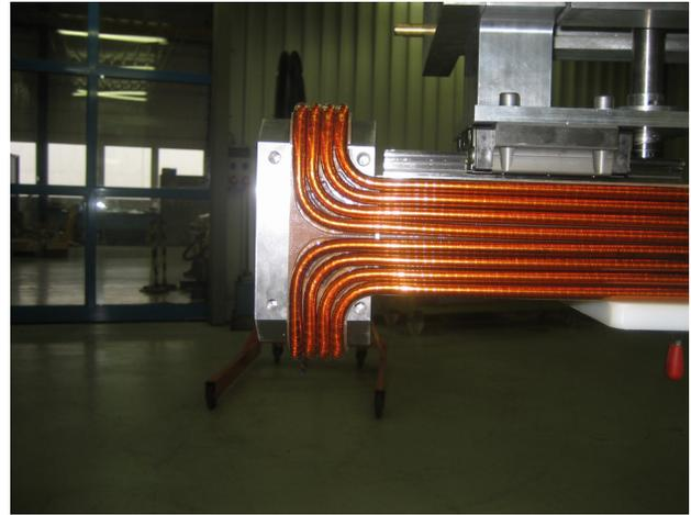
Figure 6: Picture taken during the production process of the coil head of the SIS100 pre-series dipole magnet. Winding of the stiff Nuclotron-type cable, with enhanced cross section along the small radius of curvature at the coil heads has turned out to be demanding. However the specified tolerance could be maintained.
