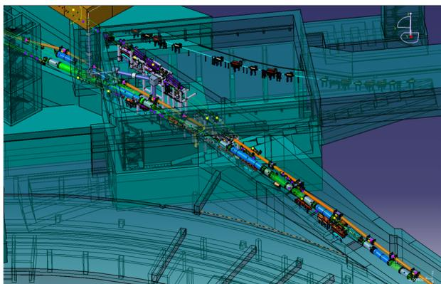
Figure 3: The FAIR high energy beam transport (HEBT) system in building 4 with vertical transfers and sloped beam lines from the underground SIS100 (down, right) to the targets on ground level (middle, up). Furthermore, shown are the two parallel beam lines of HEBT 100 and HEBT 300, on top of each other, guiding the beam to the CBM/HADES experiments situated on an intermediate level (left, up).
