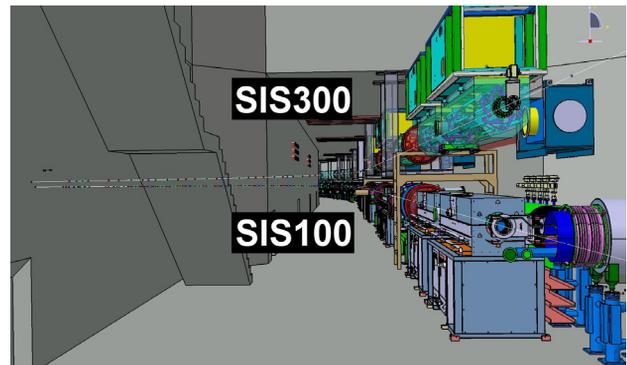
Figure 2: Front view of a straight section with the RF acceleration systems of SIS100 (below) and SIS300 (top) and the connection box of the cryogenic bypass lines (right) which bridges the warm insertions.
