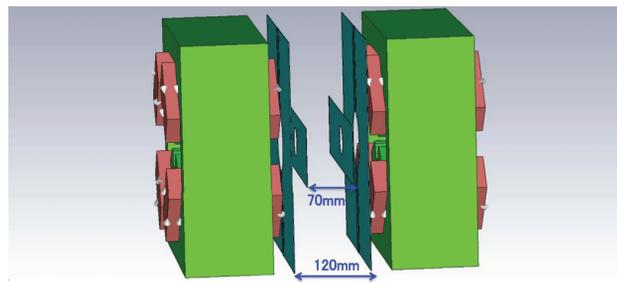
Figure 8: Simulation model of the QDM with shield.
