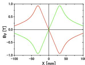
Figure 9: Magnetic field with shield at the center of the magnetic pole (red line:  $z = -150\text{mm}$ , green line:  $z = +150\text{mm}$ ).
