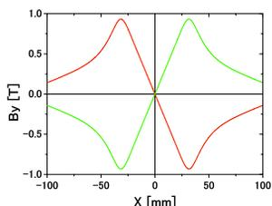
Figure 5: Magnetic field at the center of the magnetic pole (red line:  $z = -150\text{mm}$ , green line:  $z = +150\text{mm}$ ).
