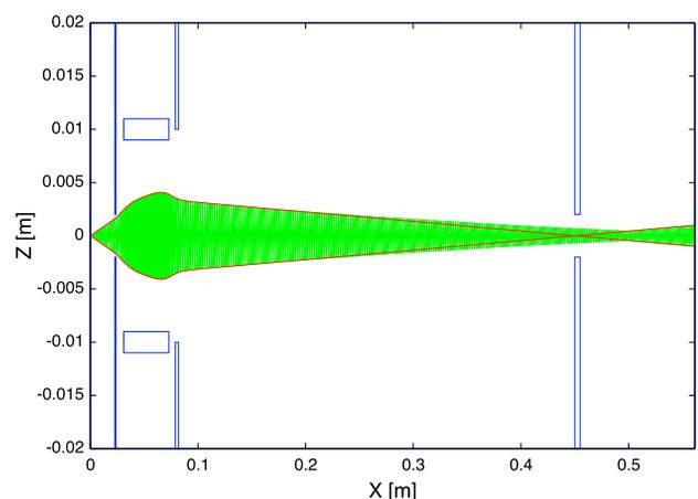
Figure 3: Electron orbit in the BSM.
