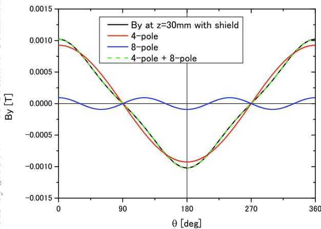
Figure 12: Superposition of the multi-pole component of the magnetic field with shield at  $z = +30\text{mm}$ .
