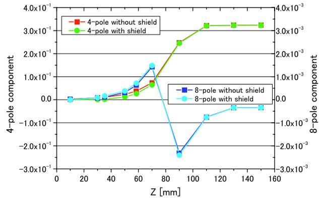
Figure 13: Multi-pole component of the magnetic field with and without shield.
