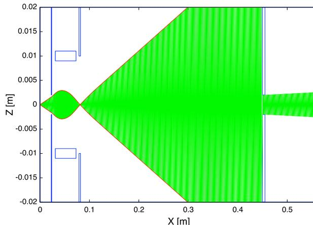
Figure 7: Electron orbit bent by the fringe field of the QDM.
