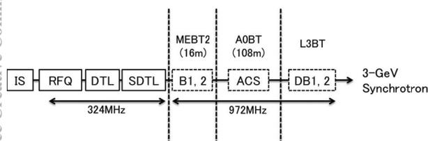
Figure 1: Diagram of J-PARC linac accelerating structures.
