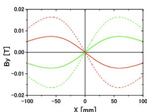
Figure 6: Magnetic field near the center of the QDM (red line:  $z = -10\text{mm}$ , green line:  $z = +10\text{mm}$ , dashed red line:  $z = -20\text{mm}$ , dashed green line:  $z = +20\text{mm}$ ).
