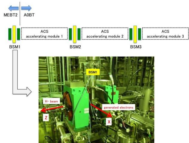
Figure 2: Installation location of the BSMs.
