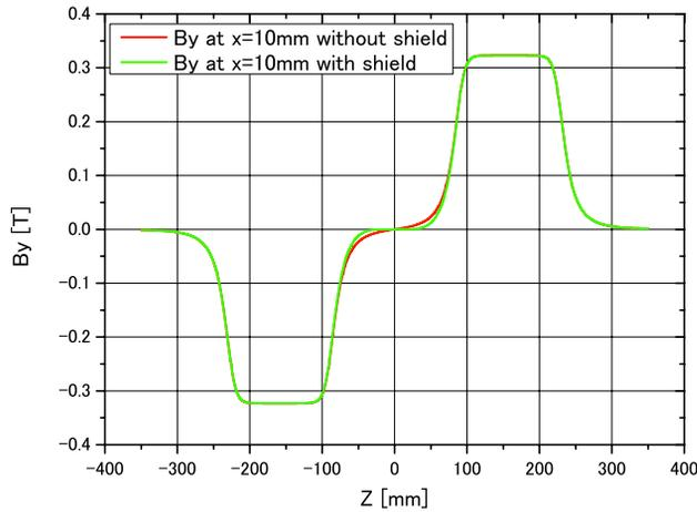
Figure 11: Magnetic field with and without shield at  $x = +10\text{mm}$ .
