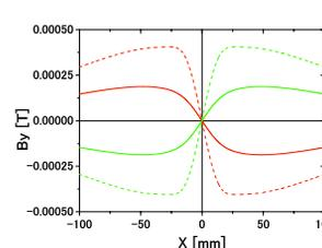
Figure 10: Magnetic field with shield near the center of the QDM (red line:  $z = -10\text{mm}$ , green line:  $z = +10\text{mm}$ , dashed red line:  $z = -20\text{mm}$ , dashed green line:  $z = +20\text{mm}$ ).
