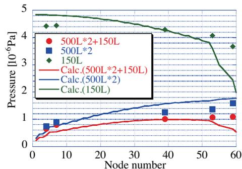
Figure 4: Comparison of pressures obtained by characteristic matrix calculation and measured pressures.
