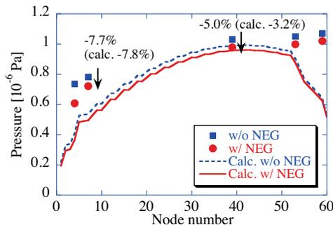
Figure 6: Pressure change between configurations with and without NEG pumps. (35-L/s NEG pumps are supposed.)
