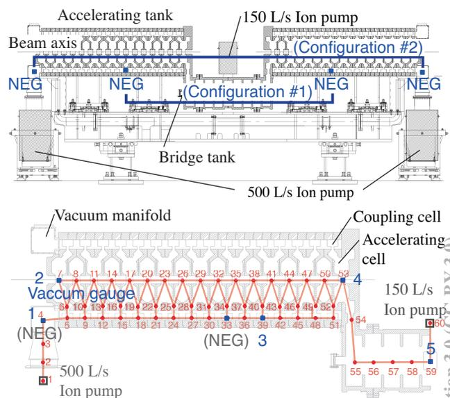
Figure 1: Configuration of NEG pumps (#1 and #2) and vacuum gauges (1-5) and diagram of the vacuum network in the ACS accelerating tank (nodes 1-60).
