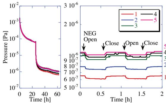
Figure 2: Evacuation curve and change in vacuum pressures caused by NEG pumps (configuration #1).
