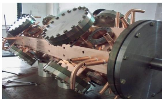
Figure 2: The fabricated 1st section of 325MHz CW RFQ.
