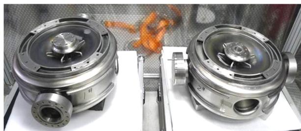
Figure 3: Two fabricated spoke012 prototype cavities.
