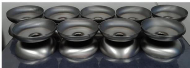
Figure 6: Cavity parts for the 650MHz Elliptical082.
