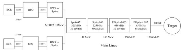
Figure 1: Layout of Chinese ADS Proton Linac.
