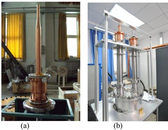
Figure 7: (a) RFQ input coupler assembly, (b) Spoke012 Cavity input coupler HP test.
