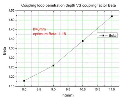
Figure 6: The calculated coupling factor under different coupling antenna loop penetration depth.
