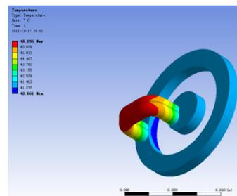
Figure 5: Simulated temperature distribution at the power level of 80 kW with a 0.4 L/min cooling water.
