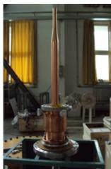
Figure 7: Fabricated window and inner conductor assembly for China ADS inject-I RFQ input coupler.
