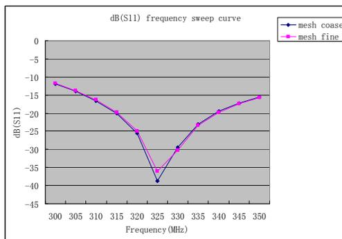
Figure 3: The reference coefficient of S11 is -37 dB at 325 MHz and the bandwidth is about 25 MHz.
