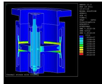
Figure 4: Simulated thermal stress distribution of RF window while 100 kW RF power passes through.
