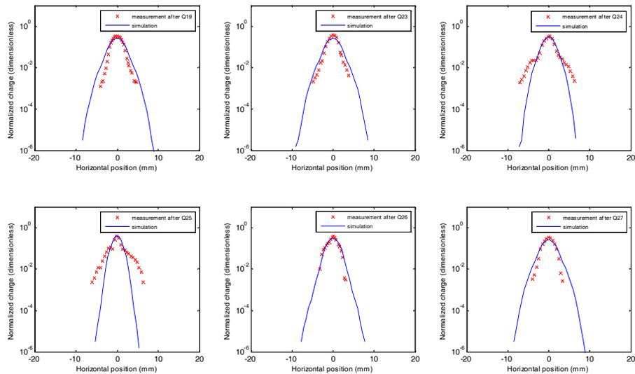
Figure 5: The horizontal profiles from measurements and simulations after Q19 Q23 Q24 Q25 Q26 Q27 for a 24.7 mA matched beam.
