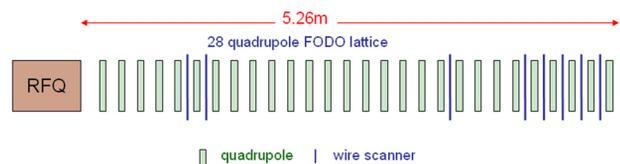
Figure 1: Block diagram of beam-core matching experiment transport line.
