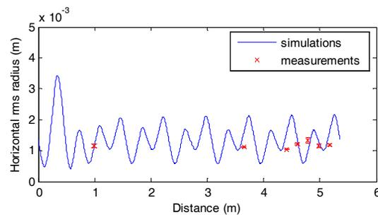
Figure 4: Horizontal rms beam size as a function of distance at a 24.7 mA matched beam.
