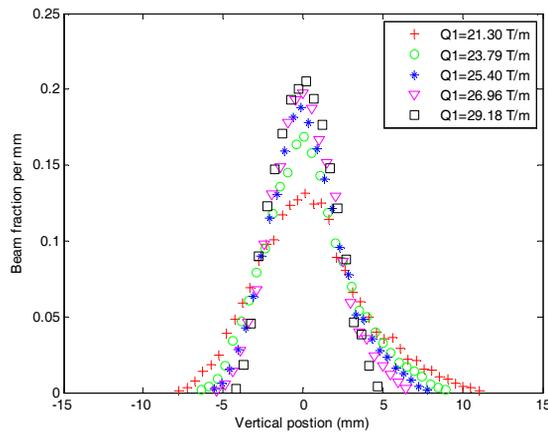
Figure 2: The beam vertical profiles measured with different focusing strength.
