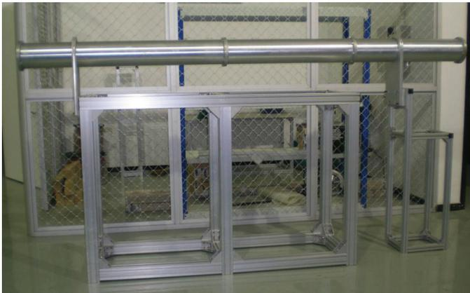
Figure 6: TOF tube for neutron imaging
