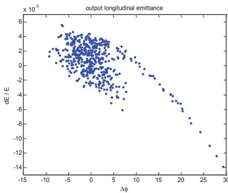
Figure 4: The beam has a long tail with non-linear effect, which lead to a low transmission efficiency of less than 80%.
