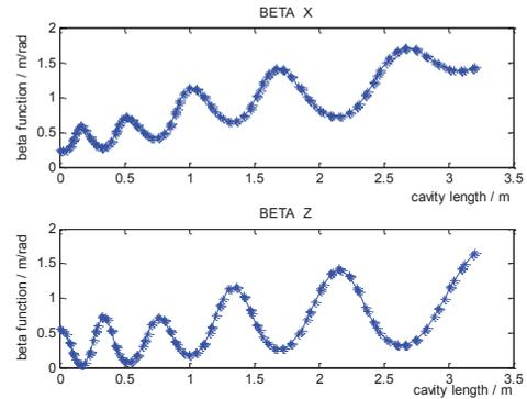
Figure 2: Betatron function in both transversal and longitudinal planes, showing excellent smoothness.
