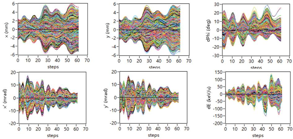
Figure 9. Six dimension beam sizes are shown as a function of cell number. One step in figures represents one cell. The beam size is controlled so well that all of 5000 particles is get through the cavity without particle lose; The longitudinal beam size and energy spread are small as well.
