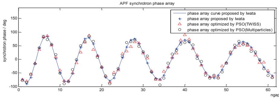
Figure 1: The general profile of synchrotron phase array generated from the formula proposed by Iwata is shown in blue curve, and phase array is shown in blue star. The red  $\Delta$  represents the synchrotron phase array optimized by PSO using TWISS transformation, black o by PSO using multiparticle track.
