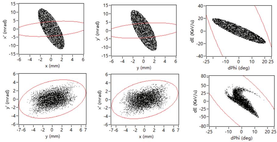
Figure 8: The emittances at input end in three phase space is shown in the upper three figures respectively, and emittances at output end is shown in lower three figures. The initial input is KV distribution.
