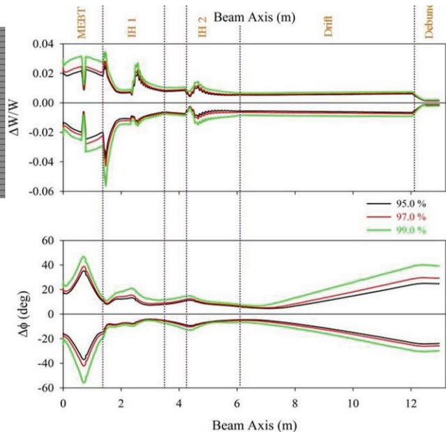
Figure 6: Longitudinal beam envelopes along the HILac.
