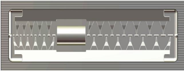
Figure 3: Cross section of IH-DTL 1.
