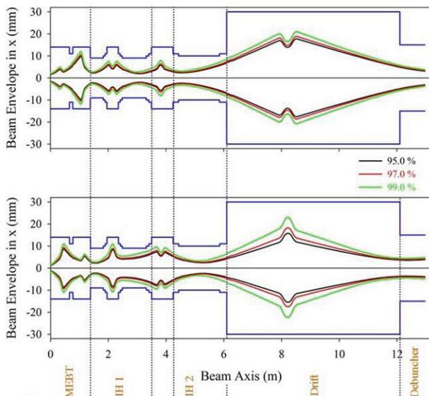
Figure 5: Transverse beam envelopes along the HILac.
