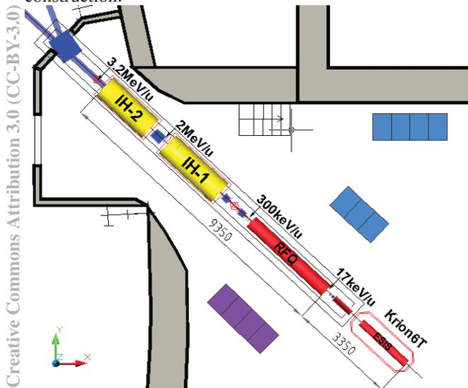
Figure 1: Layout of the heavy ion injector for NICA.
