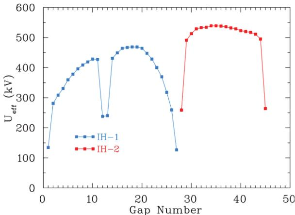
Figure 4: Effective gap voltage distribution along the IH – DTL.
