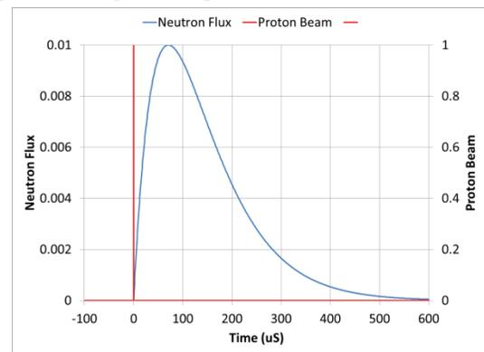
Figure 2: Target and neutron moderator response to a single proton beam pulse.
