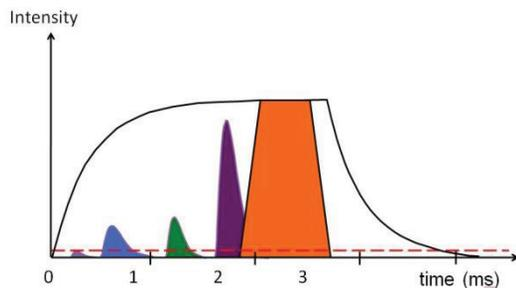
Figure 1: ESS Neutron pulse shaping concept.
