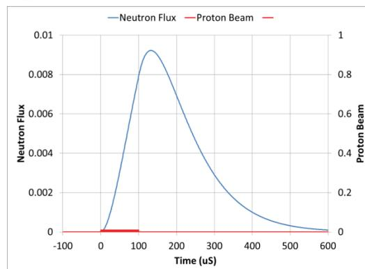
Figure 5: Target and neutron moderator response to 100 proton beam pulses.
