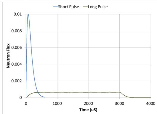
Figure 3: Target and neutron moderator response to a short and long (3 ms) proton pulse with the same number of protons per pulse.
