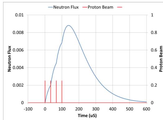
Figure 4: Target and neutron moderator response to four proton beam pulses.
