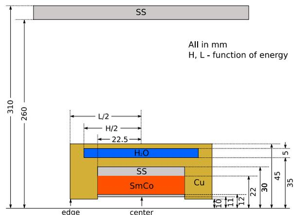
Figure 4: Computational model for the ESS DTL.
