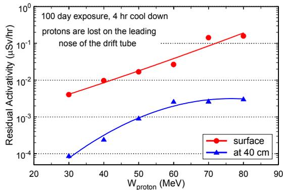
Figure 5: Residual dose rate at the surface and 40 cm from the surface of the DTL as a function of proton energy.
