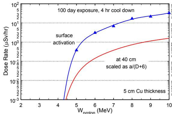
Figure 2: Expected surface dose rates and dose rates at 40 cm from the RFQ.
