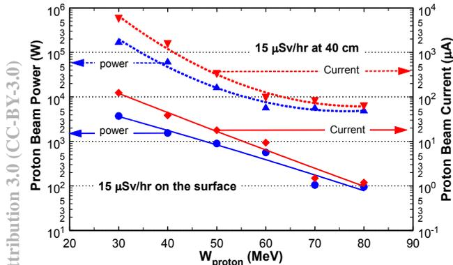
Figure 6: Beam power and current of protons lost at a point required to activate the DTL surface to 15 µSv/h and produce ambient dose rate of 15 µSv/h at 40 cm.
