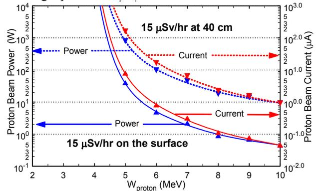
Figure 3: Power and current of lost protons required to activate the RFQ surface to 15 µSv/h and produce an ambient dose rate of 15 µSv/h at 40 cm.
