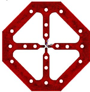
Figure 1: Typical cross section of a modern RFQ.
