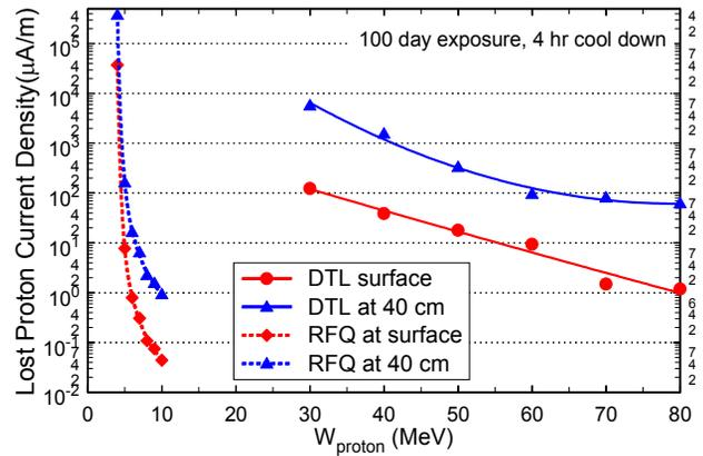
Figure 7: Average linear current density of lost protons required to activate the linac surface to 15 µSv/h and the current density required to produce an ambient dose rate of 15 µSv/h, 40 cm from the surface.
