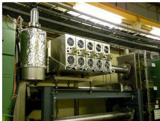
Figure 1: Prototype wideband cavity cells installed in Ring 4 of the PSB.
