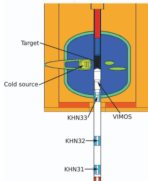
Figure 2: Schematic of the SINQ target region. The proton beam comes from the bottom.
