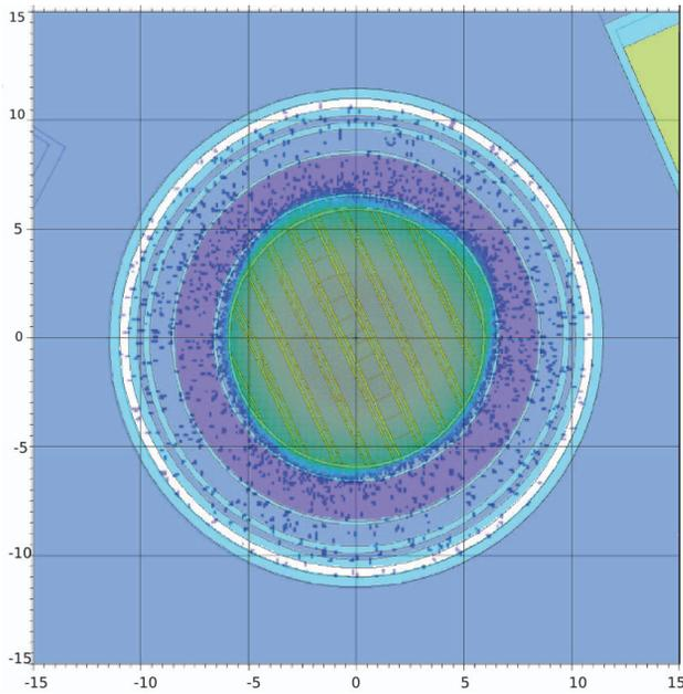
Figure 5: Beam footprint on the first row of the target tubes. For the calculation of the energy deposition the central tube was divided into 13 sections (red segments).
