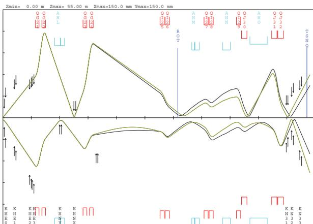
Figure 3:  $2\sigma$  beam envelope from target E to the SINQ target. Arrows represent collimators. More details are presented in the text.
