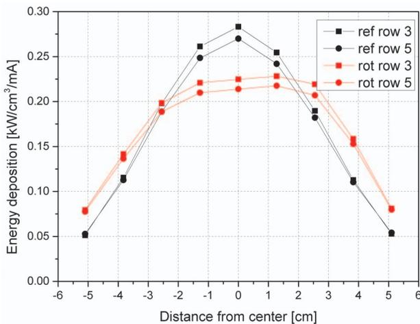
Figure 6: Energy deposition in the rods of the first two odd numbered rows for reference (black) and rotating beam.
