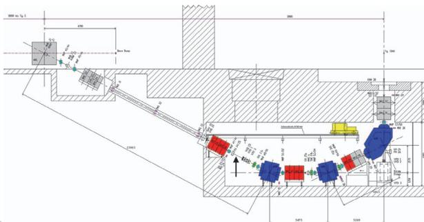
Figure 1: Layout of the SINQ beam line. The black arrow indicates the possible location of a beam rotation system.
