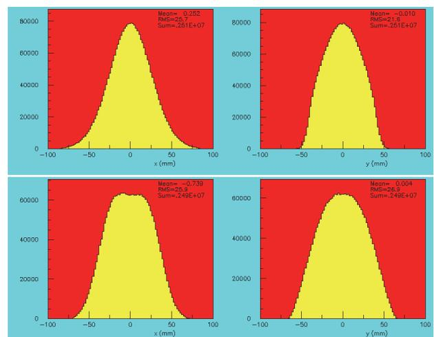
Figure 4:  $2\sigma$  Turtle simulation of the proton beam transverse distributions at the SINQ target entrance window in normal running conditions (top) and applying a beam rotation system (bottom). The coordinate system follows the Turtle convention ( $x$  is the bending plane).
