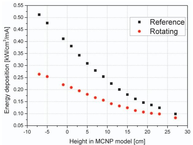
Figure 7: Energy deposition in the central section of the central odd numbered lead rods. Missing points are due to zircaloy tubes filled with probes instead of lead.
