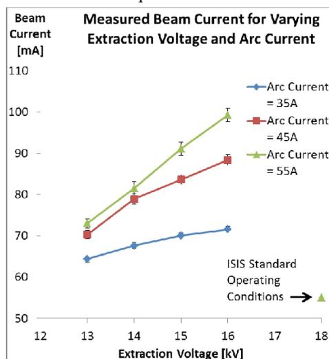
Figure 1: Development ion source beam current.
