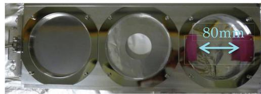
Figure 8: OTR/fluorescent screen at 350BT. Ti foil 10  $\mu$ m thick, Al foil 100  $\mu$ m thick with a 50 mm diameter hole, and fluorescent screen: Chromium doped  $Al_2O_3$  500 $\mu$ m thick, are shown from left to right.
