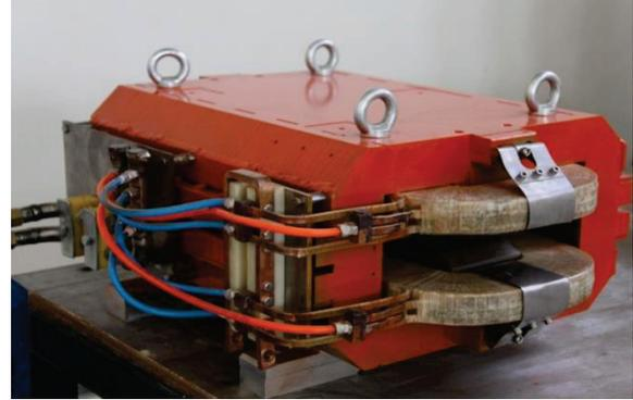
Figure 2: ILSF H-type dipole magnet.
