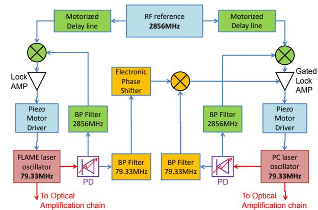
Figure 4: Sketch of the lasers synchronization scheme used in the Thomson scattering experiment.
