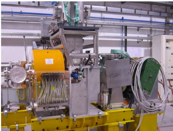
Figure 3: The Thomson scattering interaction chamber.
